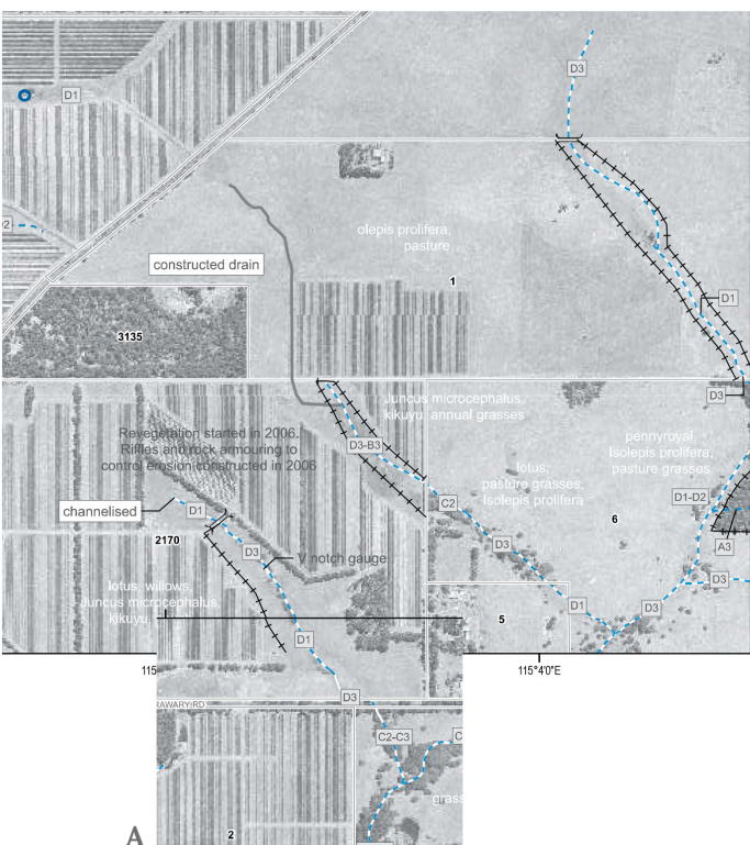
Figure 5. Comparison of revegetation over time. Image A is prior to 2009 and sourced from Boodjidup Brook Action Plan (CCCG 2009). Weightman Dam had not been constructed yet and is a bare paddock with the watercourse graded as class D3, heavily eroded. Image B is sourced from Google Maps, circa 2013–2017, the revegetation program at Weightman Dam (Figure 2, location C) had not commenced with riparian revegetation to Ullinger’s Creek line, (Figure 2, location A) newly established.
