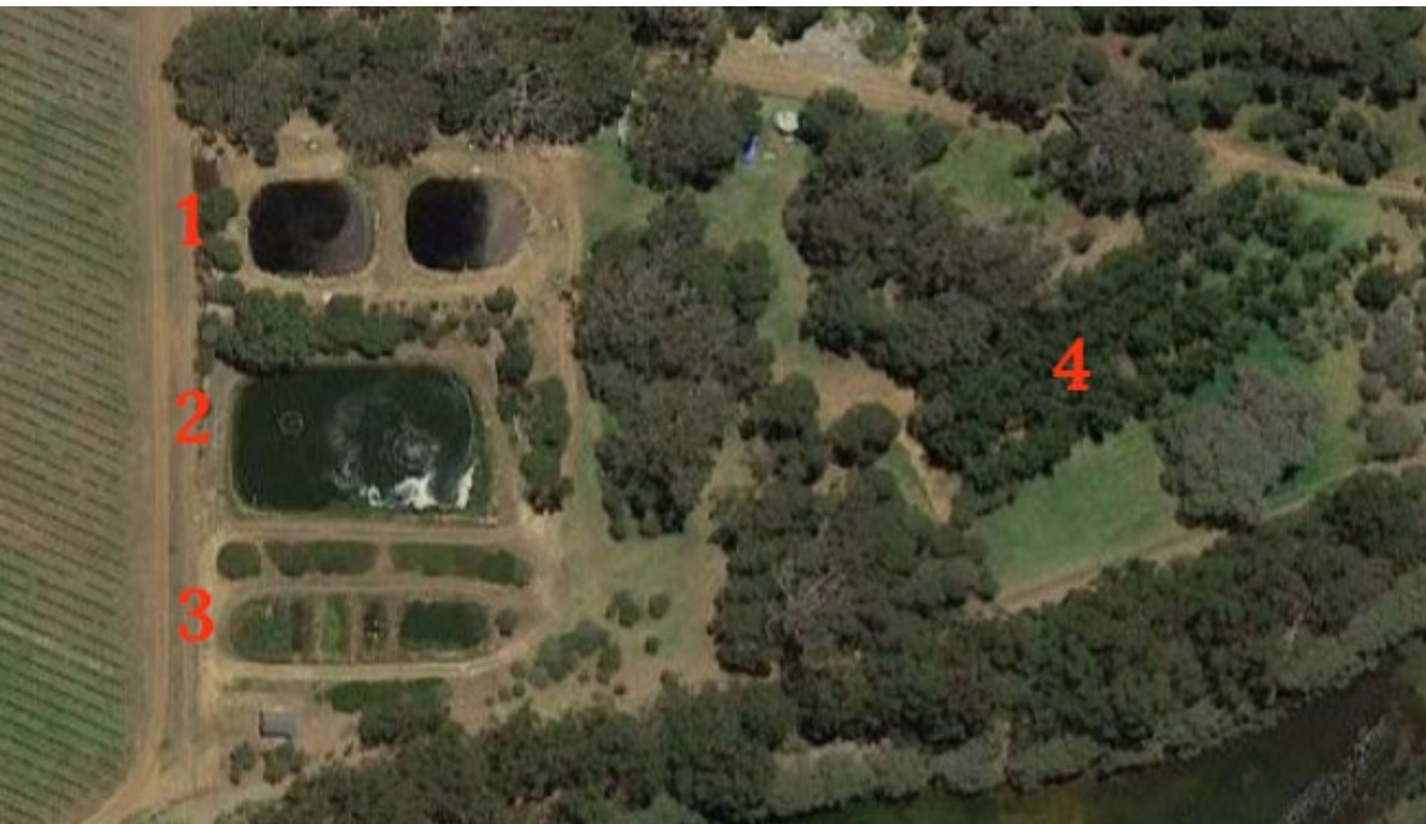
Figure 2. Cape Mentelle Vineyards' series of treatment ponds utilising gravity flow between ponds, which can be facilitated by pumps if required. Primary treatment implements sedimentation and anaerobic digestion (1) which after 30 days feeds into the secondary aeration treatment pond (2). Aeration is supplied by two pumps suspended on floating pontoons to reduce BOD. Wastewater then passes through five papyrus reed beds (3) and is finally irrigated onto an established woodlot of eastern sheoaks (4).
