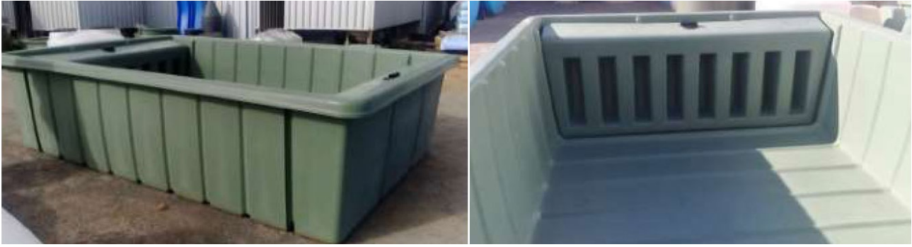
Figure 7. Reed bed pods used at Stormflower Vineyard, which are lined with a self-supporting slotted trench liner to facilitate even dispersion of wastewater to maximise interaction with reeds' root systems.
